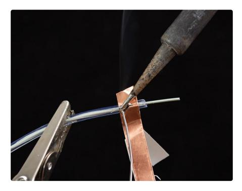
Once you've soldered your connector on, attach it to the inverter and test it, make sure the EL is glowing.
