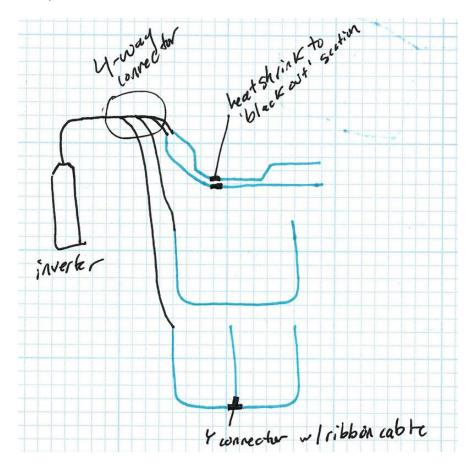
Since the pocket AA inverters can only drive 2 or 3 meters or wire maximum, its smart to keep the design short and sweet. Keep track of how long the final wire will be, add up all the segments and keep the number under 2.5m for the best look. You can also of course use a larger inverter or two inverters!
