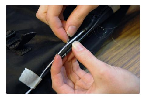
Use the needle and thread to wrap around the EL wire and tack it down, a stitch every cm is fine for long runs. We suggest grabbing plenty of material to provide a strong grip.
