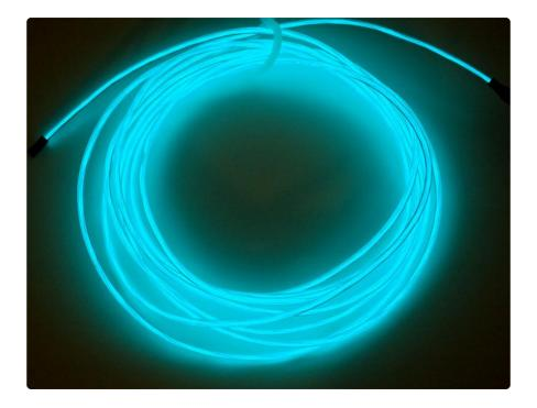
Now disconnect the wire from the inverter - never cut EL wire while its lit!
