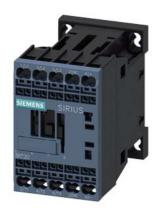
power contactor, AC-3 9 A, 4 kW / 400 V 1 NC, 24 V DC 0.7-1.25\*Us 3-pole, size S00 spring-type terminal with integrated suppressor diode spring-type terminal suitable for PLC outputs not expandable with auxiliary switch
