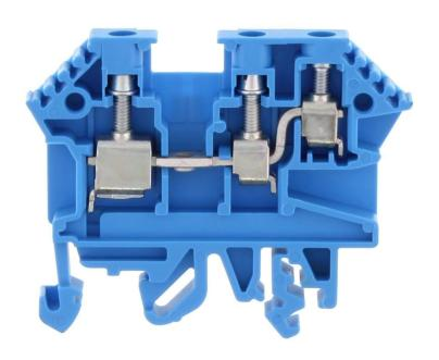
Feed-through terminal, Screw connection, Mounting type:Mounting rail TS 35/7.5 and TS 32, Rated cross-section: 4 mm², Width: 6 mm, Colour: Blue
