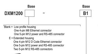
B1 = Modbus controller for data aggregation of sensors and wireless networks Power: 12-30 V DC
