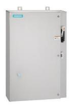
Non-reversing motor starter, Size 3, Three phase full voltage, Solid-state overload relay, OLR amp range 25-100A, Combination type, 200A fusible disconnect, 200A/250V fuse clip, Encl NEMA type 4X 304 S-Steel, Water/dust tight noncorrosive, Extra-wide enclosure
