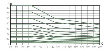
The category voltage  $(U_c)$  is consequently the maximum DC voltage which can be applied continuously at +125°C.
