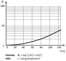
tm = maximum temperature Curve for tm = 125°C
