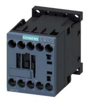
Power contactor, AC-3 9 A, 4 kW / 400 V 2 NO + 2 NC 220 V DC 4-pole Size S00 screw terminals
