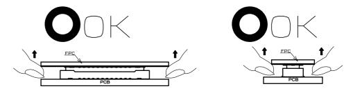
(2) IF THE CONNECTOR CANNOT BE UN-MATED PARALLEL IT CAN BE REMOVED DIAGONALLY FROM THE PITCH DIRECTION. BE CAREFUL TO DO SO SINCE THIS ACTION APPLIES STRESS ON THE CONTACT.
