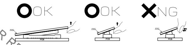
FPC IS NOT RIGID. THE CONNECTOR CAN BE BROKEN. PLEASE CHECK THE ACTION OF THE FPC TO BE USED REPEATERLY AT THE TIME OF TRIAL PRODUCTION. BE CAREFUL TO UN-MATE THEM FROM THE PITCH DIRECTION, DM THE CORNER CAN ALSO RISK TO PUTTING STRESS ON CONTACTS.
