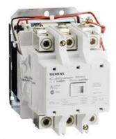
Mechanically held lighting contactor, Contactor amp rating 200A, 0 N.C. / 5 N.O. poles, 440VAC 50HZ/480VAC 60HZ coil, Non-combination type, Enclosure NEMA type (open), No enclosure
