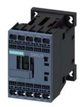
power contactor, AC-3 12 A, 5.5 kW / 400 V 1 NC, 110 V AC, 50 Hz, 120 V 60 Hz, 3-pole, Size S00 Spring-type terminal
