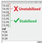
After calibration is complete, you should see readings between 9.09 - 9.1X mg/L. (only if temperature, salinity and pressure compensation are at default values)
