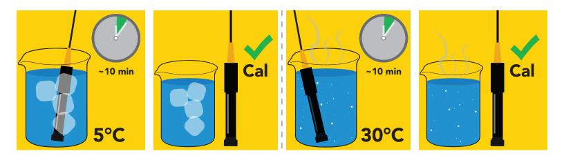
Let the probe acclimate to its operating temperature and then recalibrate. Once the probe has been calibrated at its intended operating temperature, using temperature compensation will give accurate readings.
