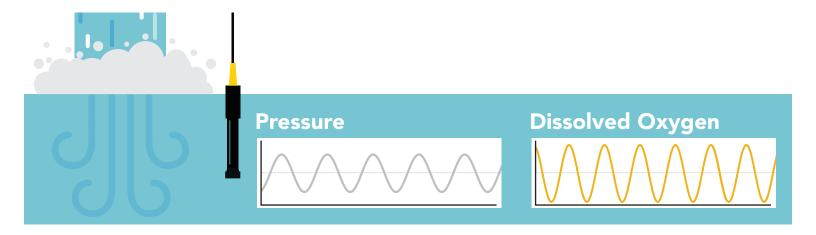
It just so happens that partial pressure of oxygen is the same in water as it is in air.
