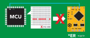
\* If one of the imported strings is not correctly entered, the device will not accept the import, respond with \*ER and reboot.
