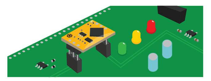
Avoid using rosin core solder. Use as little flux as possible.
