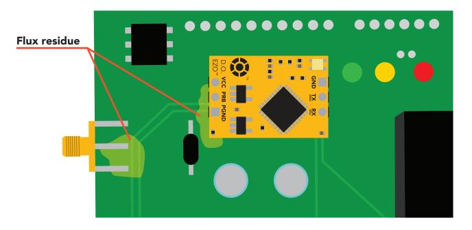
You **MUST** remove all the flux residue from your PCB after soldering.
