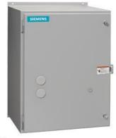
Reversing motor starter, Size 3 1/2, Three phase full voltage, Amb. compensate bimetal OLR, Contactor amp rating 115A, 110V 50Hz / 120V 60Hz coil, Non-combination type, Enclosure type 12, Dust/drip proof for indoors
