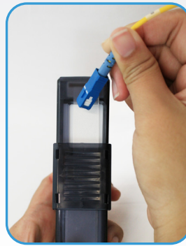
Wipe connector ferrule across cleaning surface
