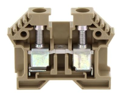
Feed-through terminal for direct mount/block variant, Screw connection, Mounting type: Mounting surface, Rated cross-section: 10 mm², Width: 8 mm, Colour: Beige
