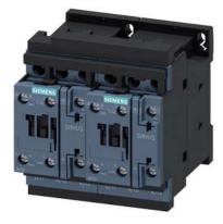
Reversing contactor assembly AC-3,18 kW/400 V,AC24V,50/60 Hz 3-pole, Size S0 screw terminal electrical and mechanical Interlock 2 NO integrated
