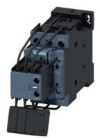
Capacitor contactor, AC-6b 25 kVAr, / 400 V 1 NO + 2 NC, 24 V DC 3-pole, Size S0 screw terminal
