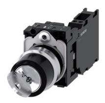
RONIS key-operated switch, 22 mm, round, metal, shiny, lock number SB30, with 2 keys, 2 switch positions O-I, latching, actuating angle 90°, 10:30h/13:30h, key removal O+I, with holder, 1 NO+1 NC, spring-type terminal, possible special locks: SB31, 421, 455 lower case
