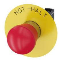
EMERGENCY STOP mushroom-type actuator, 22 mm, round, metal, shiny, red, 40 mm, positive latching, according to EN ISO 13850, pull-to-unlatch mechanism, with yellow backing plate, inscription: NOT-HALT, with holder, 1 NC, 1 NC, spring-type terminal, Z=20-unit packaging
