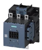
Contactor, AC-1, 275 A/690 V/40  $^\circ$ C, S6, 3-pole, 440-480 V AC/DC, with varistor, 2 NO+2 NC, Connection rail/ screw terminal
