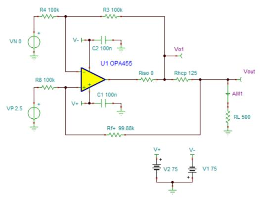
Figure 3-1. Practical, 20-mA, Improved Howland Current-Pump Circuit
