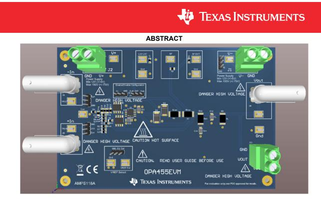
This user's guide describes the characteristics, operation, and use of the evaluation module (EVM) for the OPA455. The EVM is designed to evaluate the performance of the devices in both single and dual-supply configurations. This document also includes the schematic, printed circuit board (PCB) layout, and a bill of materials (BOM). Throughout this document the terms *evaluation board*, *evaluation module*, and *EVM* are synonymous with OPA455EVM.
