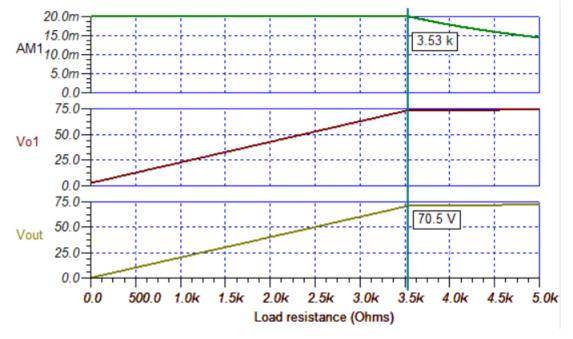
Figure 3-2. Improved Howland Current Pump Output-Voltage Compliance Range
