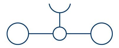
Feed-through terminal for direct mount, Tension-spring connection, Mounting type: Mounting surface, Rated cross-section: 2.5 mm<sup>2</sup>, Width: 5.1 mm, Colour: Green
