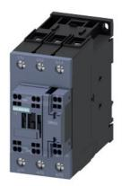
power contactor, AC-3 51 A, 22 kW / 400 V 1 NO + 1 NC, 20-33 V AC / DC 3-pole, size S2, spring-loaded terminal
