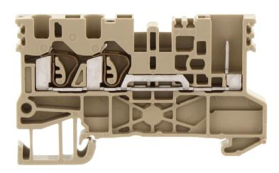
Feed-through terminal, Tension-spring connection, Mounting type: Mounting rail TS 35/7.5, Rated cross-section: 2.5 mm², Width: 5.1 mm, Colour: Beige
