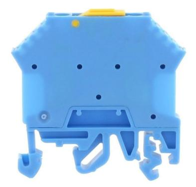
Disconnect terminal, Screw connection, Mounting type:Mounting rail TS 35/7.5 and TS 32, Rated cross-section: 2.5 mm<sup>2</sup>, Width: 6 mm, Colour: Blue
