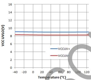
Figure 24. VCC UVLO vs. Temperature
