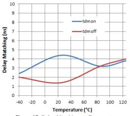
Figure 15. Delay Matching vs. Temperature
