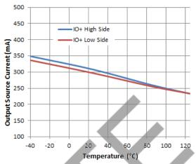
Figure 17. Output Source Current vs. Temperature
