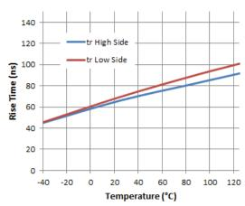
Figure 9. Rise Time vs. Temperature
