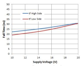
Figure 10. Fall Time vs. Supply Voltage
