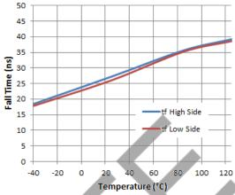
Figure 11. Fall Time vs. Temperature
