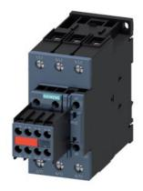
Power contactor, AC-3 80 A, 37 kW / 400 V 2 NO + 2 NC, 20-33 V AC/DC with varistor 3-pole, size S2 screw terminals Perm. mounted auxiliary switch
