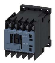
power contactor, AC-3 12 A, 5.5 kW / 400 V 1 NO, 24 V DC 0.7-1.25\* US, with suppressor diode integrated 3-pole, size S00 ring cable lug connection suitable for PLC outputs not expandable with auxiliary switch
