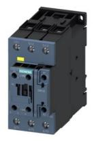
contactor, AC-3, 40 A/400 V/60 °C, S2, 3-pole, 175-280 V AC/DC, F-PLC-IN, with varistor, 1 NC, screw terminal
