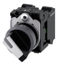
Selector switch, illuminable, 22 mm, round, plastic with metal front ring, white, selector switch, short, 2 switch positions O-I, latching, actuating angle 90°, 10:30h/13:30h, with holder, 1 NO, 1 NC, spring-type terminal, with laser labeling, inscription or symbol Customer-specific selection with SIRIUS ACT configurator (CIN)
