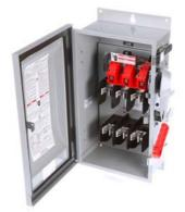
Siemens Low Voltage Circuit Protection Heavy Duty Safety Switches. Type: ENCLOSED, SAFETY SWITCH Std: UL V. Rating: 240V A. Rating: 100A Wattage: 3W No. Of Poles: 3P F. Rating: 60Hz Action: SINGLE THROW Material: 304SS Enclosure: TYPE 12. 2-3 point mounting holes. Insulation: YES O. Cycles: 10000 O. Temperature: (-20F-120F) AMBIENT TEMPERATURE Environmental Conditions: INDUSTRIAL
