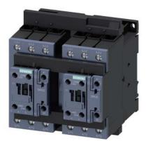
Reversing contactor assembly AC-3, 30 kW/400 V, AC/DC 20-33V 3-pole, Size S2 screw terminal electrical and mechanical Interlock 2 NO integrated
