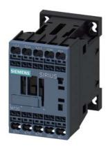
power contactor, AC-3 12 A, 5.5 kW / 400 V 1 NC, 110 V DC 0.7-1.25\*US with integrated suppressor diode 3-pole, size S00 spring-type terminal suitable for PLC outputs not expandable with auxiliary switch
