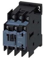
Power contactor, AC-3 38 A, 18.5 kW / 400 V 1 NO + 1 NC, 220 V AC 50 Hz, 240 V, 60Hz, 3-pole, size S0 ring cable lug connection
