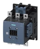
power contactor, AC-3 265 A, 132 kW / 400 V AC (50-60 Hz) / DC operation 200-277 V AC/DC auxiliary contacts 2 NO + 2 NC 3-pole, frame size S10 busbar connections drive: electronic with PLC interface 24 V DC spring-loaded terminal
