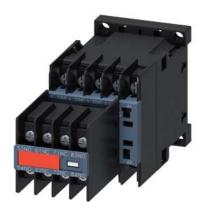
Contactor relay, 6 NO + 2 NC, 110 V AC 50 Hz / 120 V 60 Hz, Size S00, Ring cable lug connection, Captive auxiliary switch,
