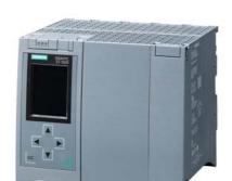
SIMATIC S7-1500F, CPU 1518F-4 PN/DP, central processing unit with 9 MB work memory for program and 60 MB for data, 1st interface: PROFINET IRT with 2-port switch, 2nd interface: PROFINET RT, 3rd interface: PROFINET basic services, 4th interface: PROFIBUS, 1 ns bit-performance, SIMATIC Memory Card required
