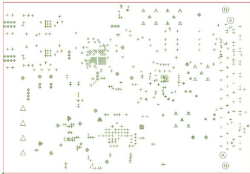
Figure 35. EVAL-ADAQ23876FMCZ and EVAL-ADAQ23878FMCZ Board Drill Chart and Size 69 mm × 100.5 mm
