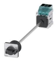
Load disconnector 3LD3, lu 40 A Main switch 3-pole Rated operating capacity at AC-23 A at 400 V 18.5 kW floor mounting Basic switch with door coupling Central hole mounting 22.5mm Toggle drive black 48x48 mm with auxiliary switch 1OE + 1S
