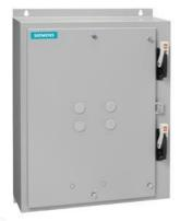
Duplex starter w/o alternator Size 1 Three phase full voltage Solid-state overload relay OLR amp range 10-40A Combination type Two 30A disconnect switches Encl NEMA type 4X 304 S. Steel Water/dust tight noncorrosive
