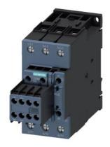
Power contactor, AC-3 65 A, 30 kW / 400 V 2 NO + 2 NC, AC / DC 20-33 V, with varistor 3-pole, size S2 screw terminals
