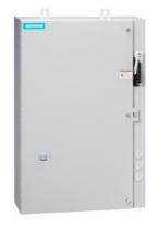
Non-reversing motor starter, Size 2, Three phase full voltage, Solid-state overload relay, OLR amp range 13-52A, 24VAC 50-60Hz coil, Combination type, 50A circuit breaker, Enclosure NEMA type 4/12, Water/dust tight for outdoors, Extra-wide enclosure
