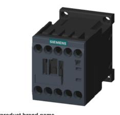
Power contactor, AC-3 12 A, 5.5 kW / 400 V 1 NC, 24 V AC, 50 / 60 Hz 3-pole, Size S00 screw terminal
