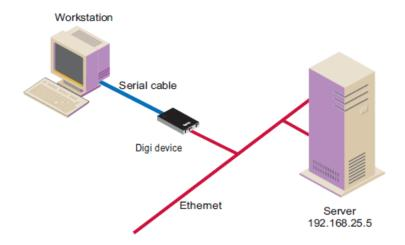
In Diagram A, the Digi device replaces a modem connected to a workstation running an application. The Digi device allows you to use software applications without modification by responding to all the AT commands configured in the workstation application. The Digi device connects to the IP Address of the server when you issue the following command:
