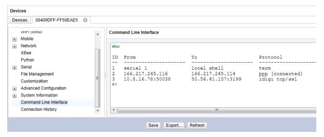
3. Enter commands following the command syntax as shown in this Command Reference. The example shows entering the **who** command and its output.
