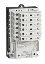
Electrically held lighting contactor, (convertible to mech. held), Amp rating 30A (tungsten 20A), 6 N.C. / 1 N.O. poles, 277V 60Hz / 240V 50Hz coil, Non-combination type, Enclosure NEMA type (open), No enclosure
