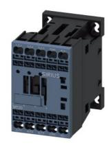
Power contactor, AC-3 7 A, 3 kW / 400 V 1 NC, 24 V DC communication-capable, 3-pole, Size S00, Spring-type terminal
