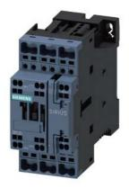
power contactor, AC-3 17 A, 7.5 kW / 400 V 1 NO + 1 NC, 48 V DC, 3-pole, Size S0 Spring-type terminal
