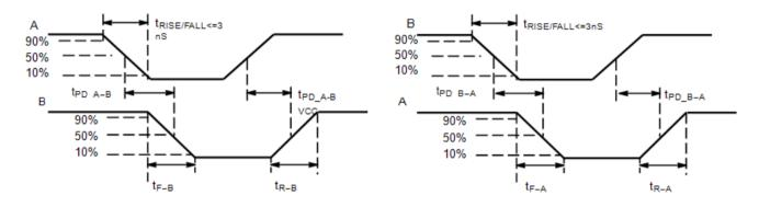
Figure 4. Definition of Timing Specification Parameters
