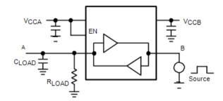
Figure 2. Driving A Test Circuit
