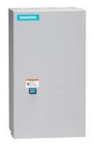
Reversing motor starter, Size 3, Three phase full voltage, Solid-state overload relay, OLR amp range 25-100A, 24VAC 50-60Hz coil, Noncombination type, Enclosure type 1, Indoor general purpose use, Standard width enclosure
