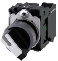
Selector switch, illuminable, 22 mm, round, plastic with metal front ring, white, selector switch, short, 2 switch positions O-I, latching, actuating angle 90°, 10:30h/13:30h, with holder, 1 NO, spring-type terminal, with laser labeling, inscription or symbol Customer-specific selection with SIRIUS ACT configurator (CIN)
