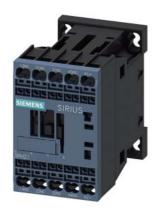
Coupling contactor relay, 2 NO + 2 NC, 110 V DC, 0.7  $\dots$  1.25\* US, with integrated suppressor diode, Size S00, Spring-type terminal suitable for PLC outputs
